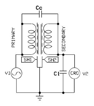
Primary are shorted on input side Secondary are shorted on output side. Both input and output shields are grounded
